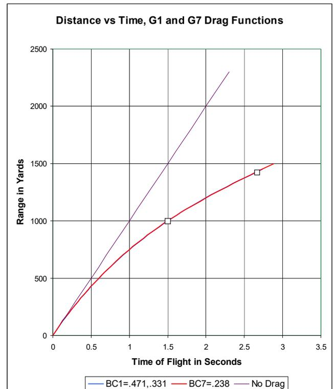
After adding the stepped change in the G1 ballistic coefficient, the blue G1 curve is obscured by the red G7 curve out to approximately 1500 yards. If you want your predictions to reliably extend to even longer ranges, then you must test at longer ranges and add the additional trued steps to your ballistic coefficients.
