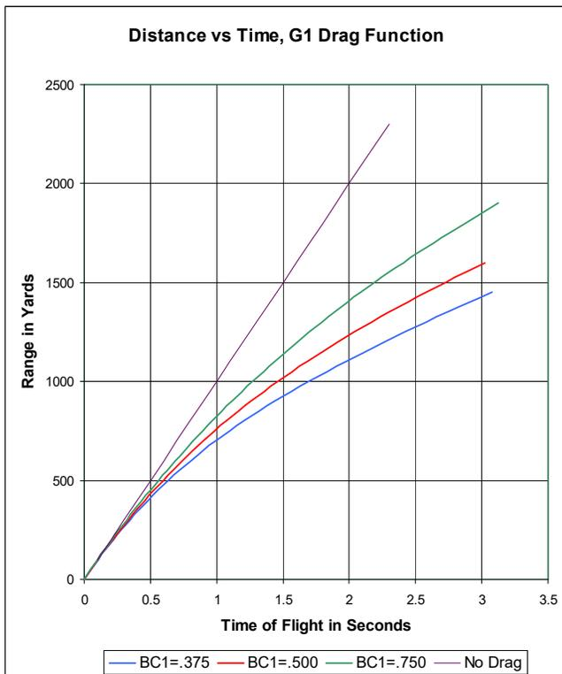
Here are the distance-versus-time curves for three bullets. All have a muzzle velocity of 3000 feet per second. The nice thin black line at the top of the cluster is our old friend with no air drag. The lower curves are those predicted using the common G1 drag function with ballistic
