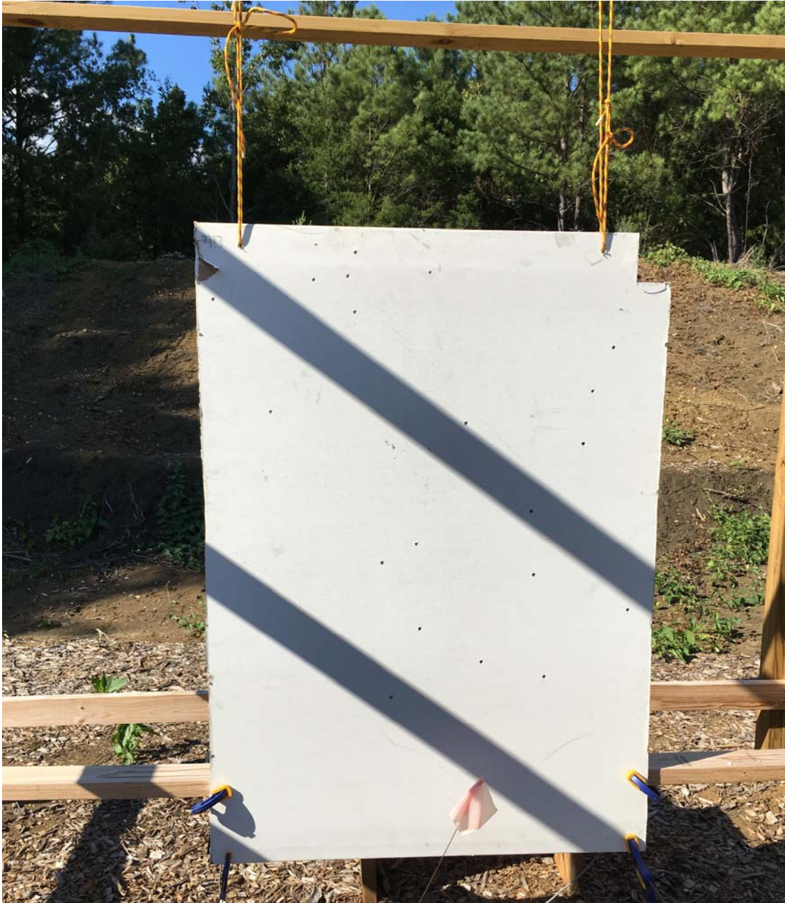
A piece of drywall material is hung in the frame to detect subsonic bullets. Two microphones are mounted behind the lower corners of the sheet.
